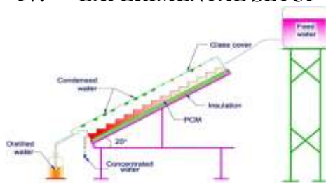
Fig.1 Schematic diagram of experimental setup of solar still with PCM.
